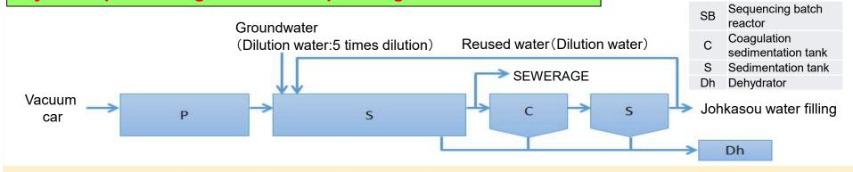
The suspended Omihachiman Night Soil Treatment Plant was designed and repaired so as to operate at a low cost. As compared with the standard treatment method, it uses less diluted water, is more compact, saves power and uses the SBR method which is superior in denitrification.
